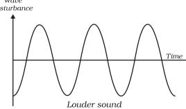
**Fig. 11.8:** Soft sound has small amplitude and louder sound has large amplitude.
