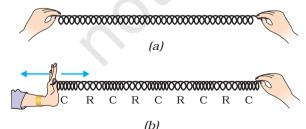
Fig. 11.5: Longitudinal wave in a slinky.
