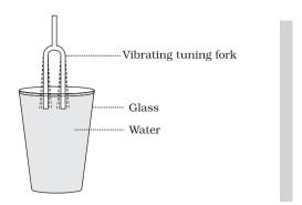
Fig. 11.3: Both the prongs of the vibrating tuning fork dipped in water
