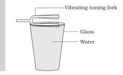
Fig. 11.2: One of the prongs of the vibrating tuning fork touching the water surface.
