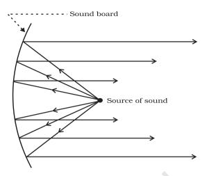
Fig. 11.13: Sound board used in a big hall.
